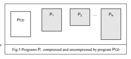
compression program PCD, which may or may not be memory resident, the compression code is necessary only in one instance and the self-replicating code is unnecessary (Fig.5). It can be seen, that the programs  $P_1$ - $P_N$ , on which the compression program PCD was applied, contain no extraneous code.
